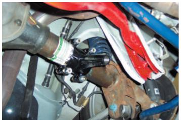
NOTE: Do to slight variations in the Mustang chassis assembly and welding at the factory it may be necessary to grind some clearance in the passenger side chassis holes. If this appears to be the case, you are welcome to call us for guidance.
