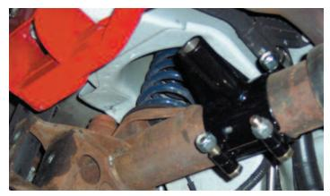
4c) Next position the passenger side axle tube mount so that it points to the rear and downward at about the 4 0-clock position. Snug the nuts and bolts but leave them loose enough so you can slide the axle tube mount from side to side and rotate it on the axle tube. You will note that the axle tube mounts movement is limited by the slot which fits around the axle tube breather.
