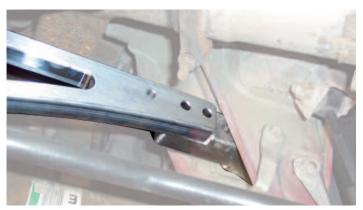
NOTE: Do to slight variations in the Mustang chassis assembly and welding at the factory it may be necessary to grind some clearance in the passenger side chassis holes. If this appears to be the case, you are welcome to call us for guidance.
