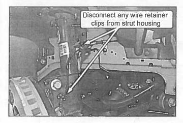
Disconnect the front stabilizer bar link from the strut housing. Use a 17mm wrench on the flats of the stud to stop it from rotating and an 18mm socket to remove the nut.
